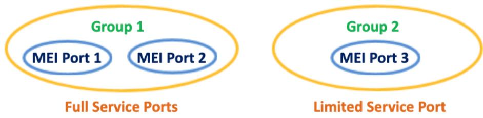
For this example, the group 2 is set up to not cleanup on disconnect. But, the group 1 is set up to cleanup on disconnect.
