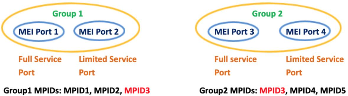
For this example, both groups are set up to cleanup on disconnect. MPID3 is shared on both groups. Port 1 and 3 are full service ports. Port 2 and 4 are limited service ports. Please note that in this setup, MPIDs 1, 2, 4 and 5 will not benefit from redundancy. Firms are encouraged to consider such disadvantages with the setup they are requesting.
